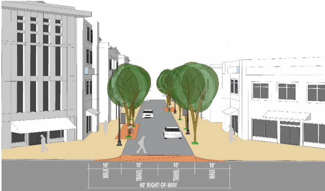
Figure 8 Typical Cross Section for a Woonerf
