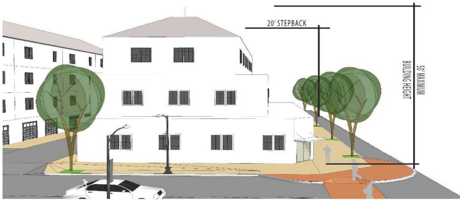
Figure 1 Building Stepbacks and Setbacks
