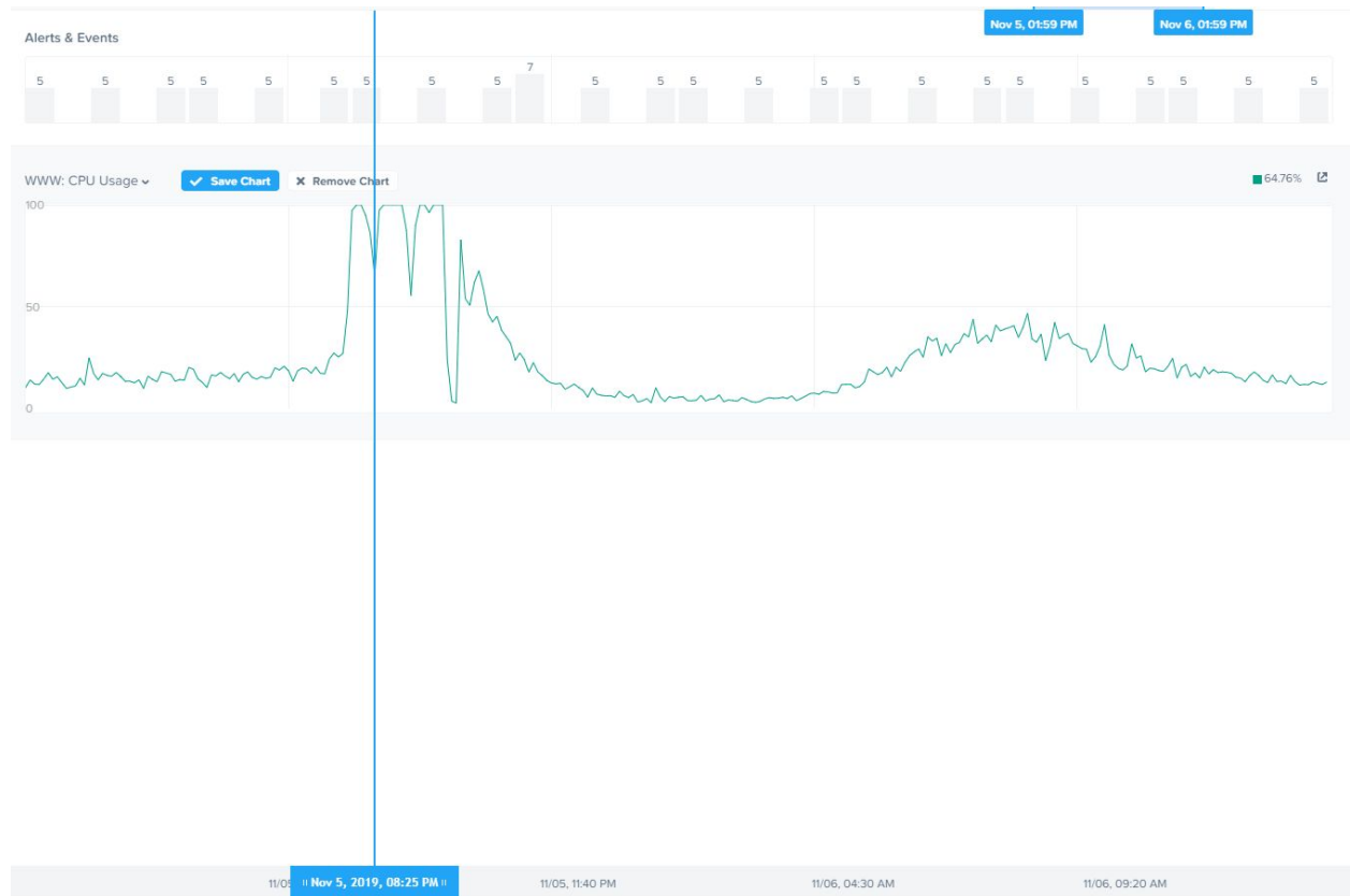
Figure c. Webserver is again rebooted at approx 9:05pm. The purpose of this reboot is too add more memory in an attempt to alleviate the CPU pressure. Again, the usage spikes after coming online.
