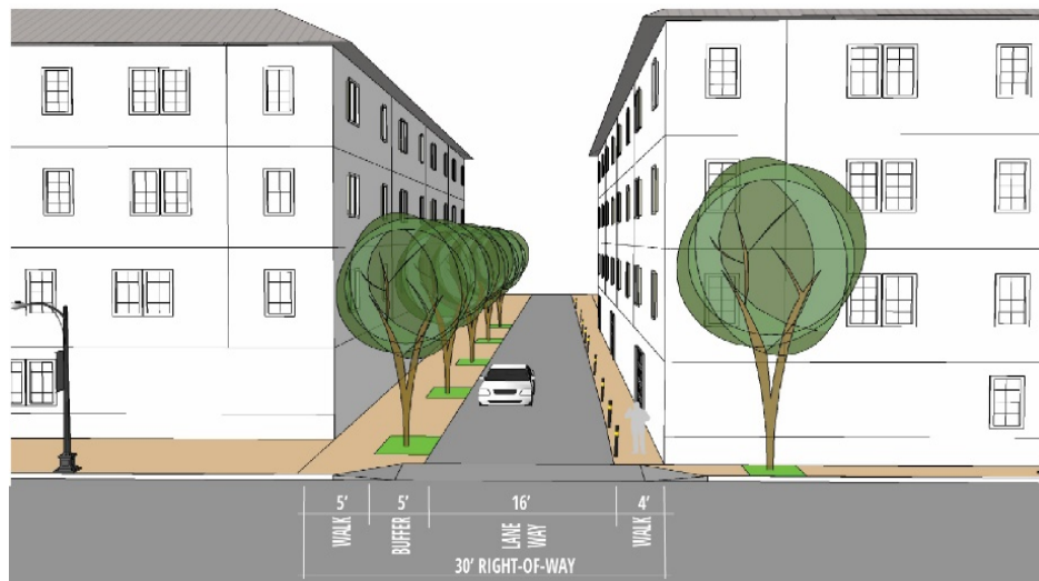
Figure 7 Typical Cross Section for a Laneway
