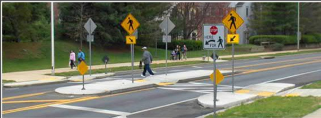
MID-BLOCK CROSSING WITH CENTER PEDESTRIAN REFUGE
