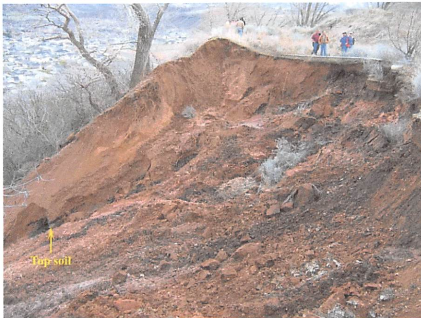
Figure 6. View to the southeast showing landslide main scarp and fill placed on the upper slope. Near the left edge of the photo, black top soil at the base of the scarp (arrow) underlying the brown fill is evident and indicates the original slope surface.
