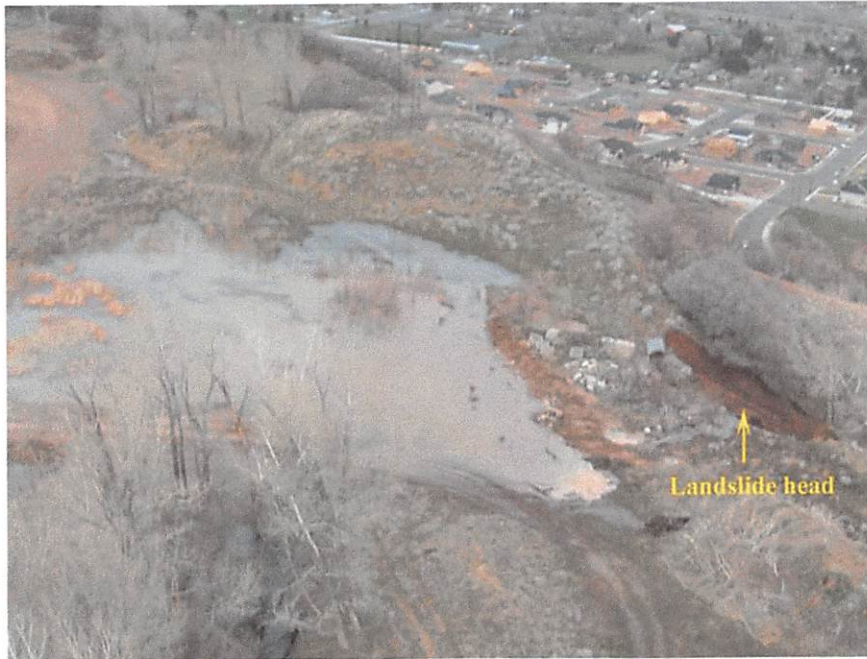
Figure 5. View looking northwest at the pond in the gravel pit and the landslide head (arrow). A berm was placed between the pond and the landslide to prevent water from flowing onto the landslide. Photo taken on the morning of April 10, 2005, by Davis County Sheriff's Office personnel.
