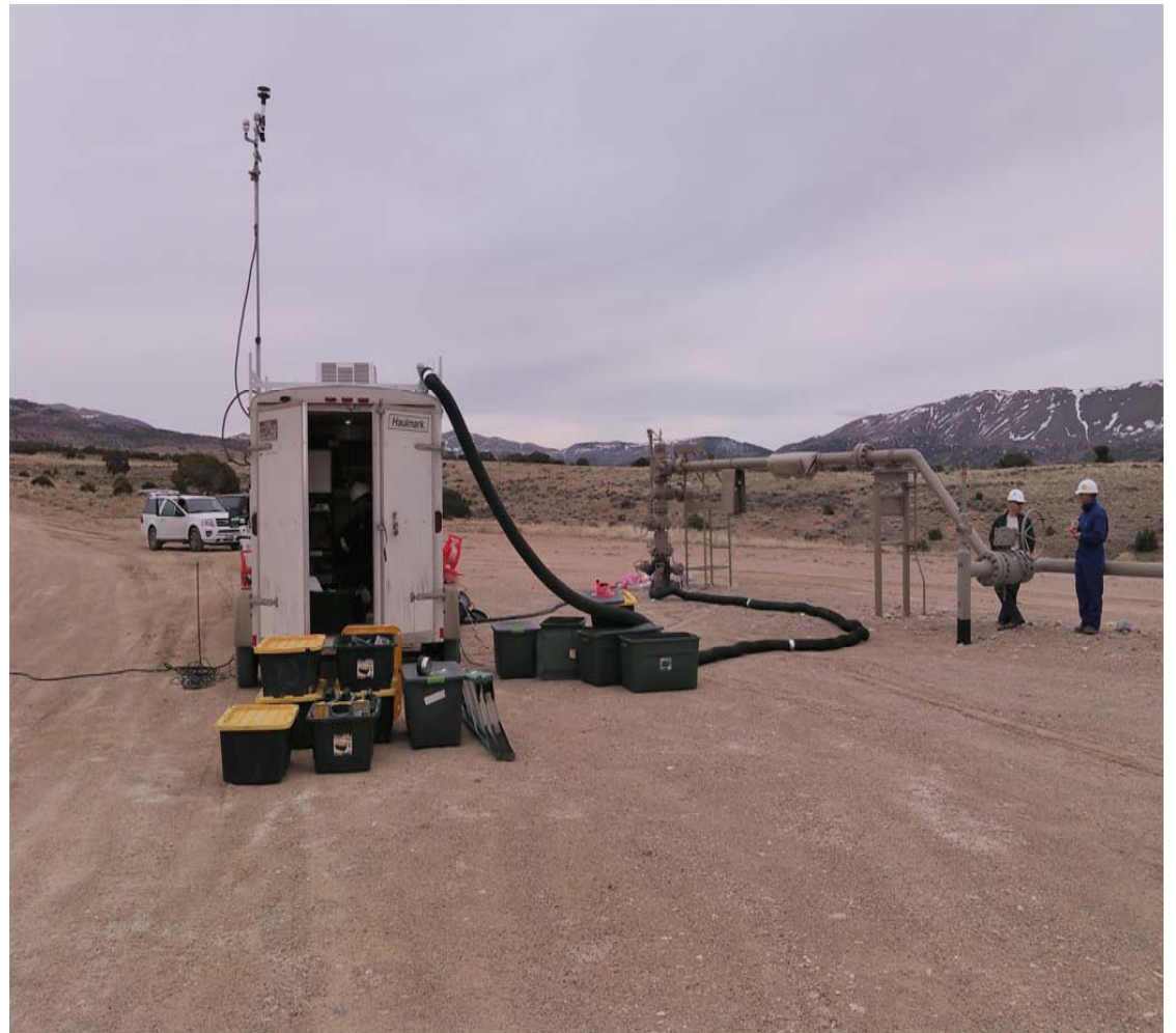
Direct emission sampling (high-flow)
