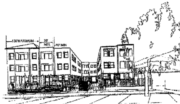
Typical Roofline Breaks
