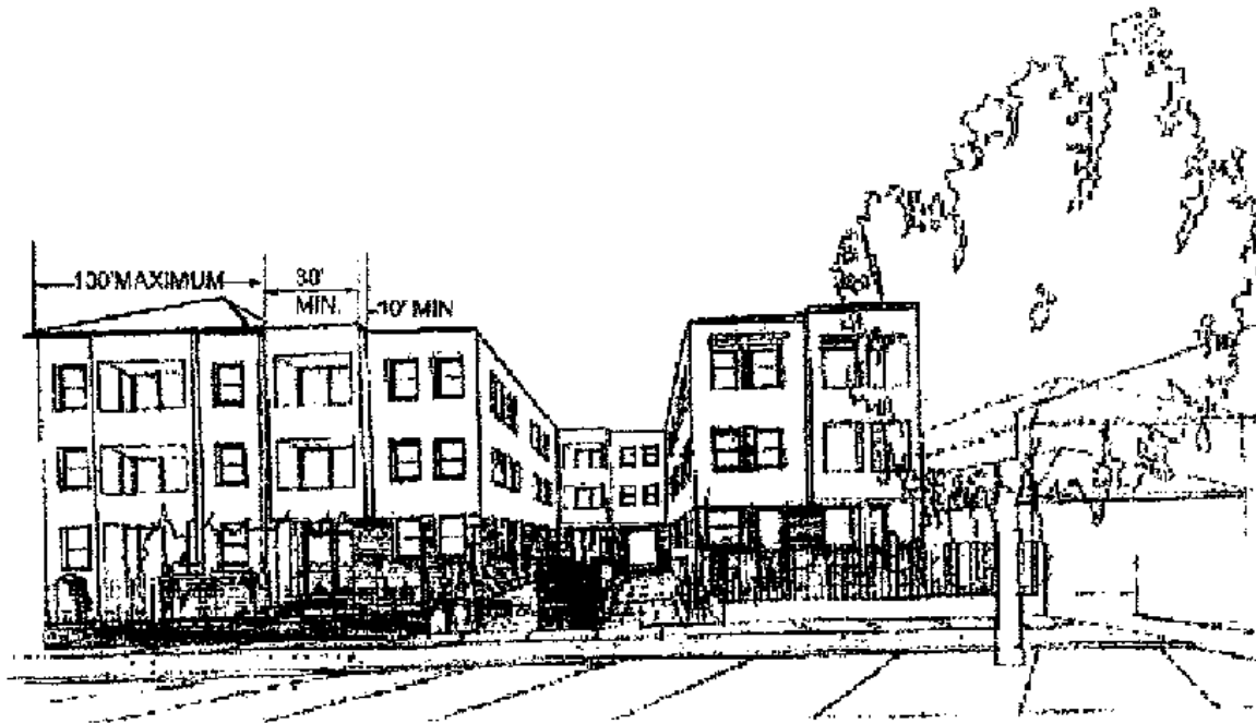
Typical Roofline Breaks
