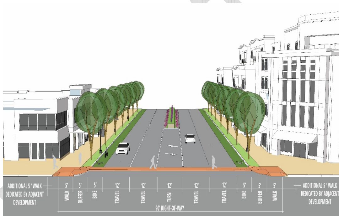
Figure 4 Typical Cross Section for Richmond Boulevard
