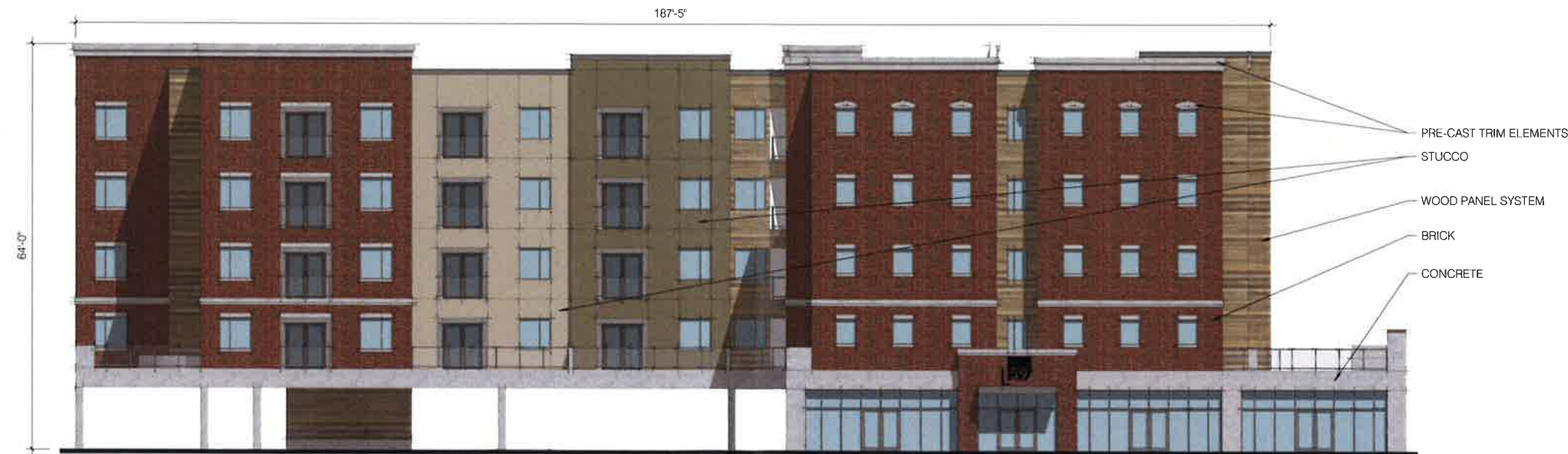
2 MAIN BUILDING WEST ELEVATION AE202 SCALE: 3/32" = 1'-0"
