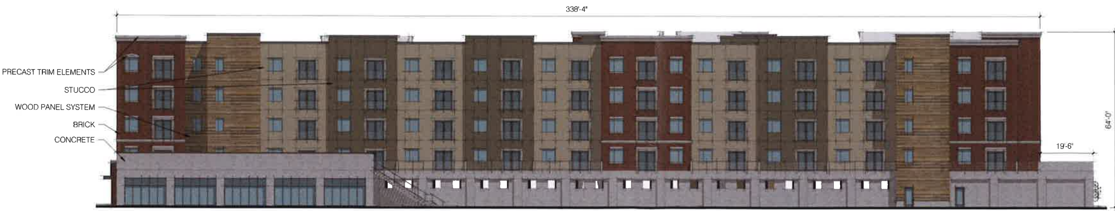
2 MAIN BUILDING SOUTH ELEVATION AE201 SCALE: 1/16" = 1'-0"
