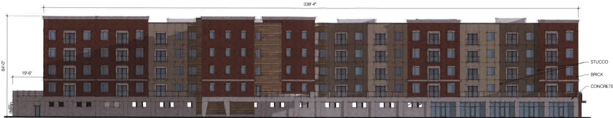
1 MAIN BUILDING NORTH ELEVATION AE201 SCALE: 1/16" = 1'-0"
