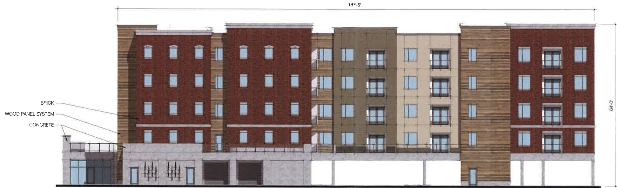
1 MAIN BUILDING EAST ELEVATION AE202 SCALE: 3/32" = 1'-0"
