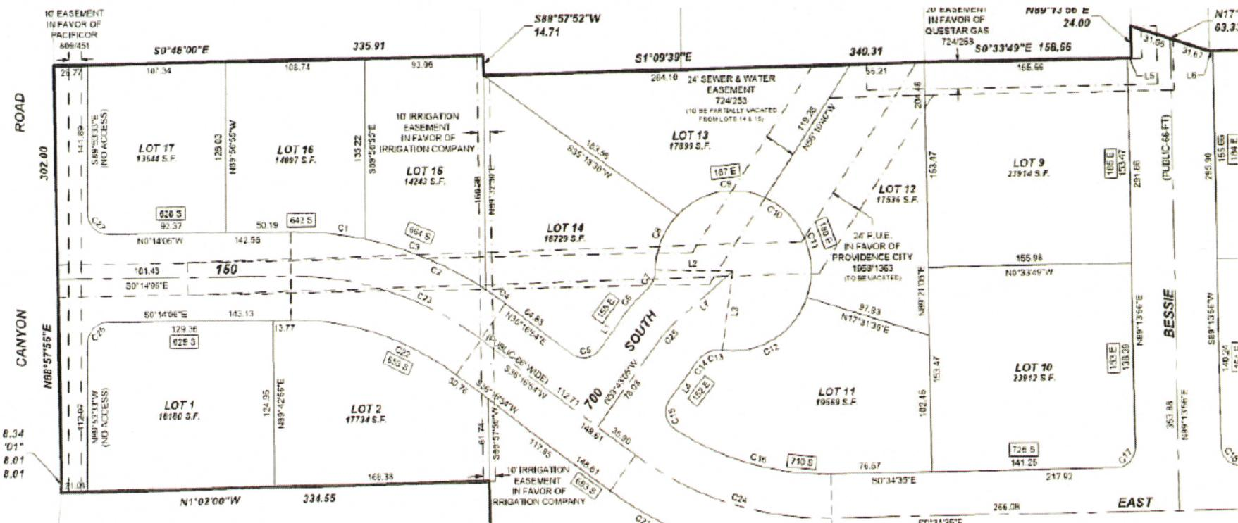
The existing portion of the easement shown in the proposed Lot 13 will remain. The portion of this easement shown in Lots 14 and 15 and extending into the proposed 150 East is proposed be vacated.
