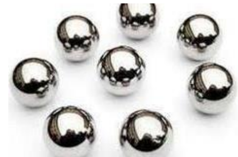
Steel Balls used to crush concrete
