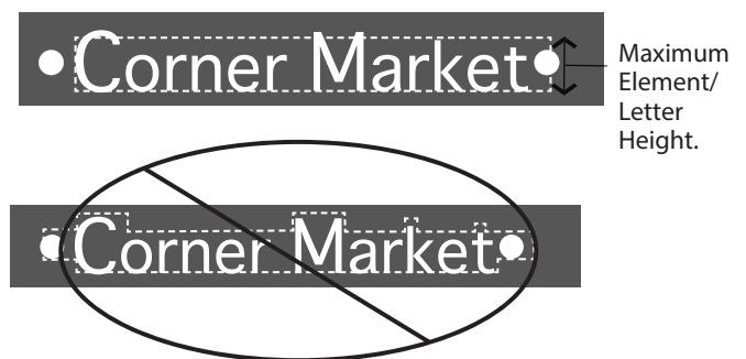
Figure 9.3 (2). Measuring Wall Signs.
