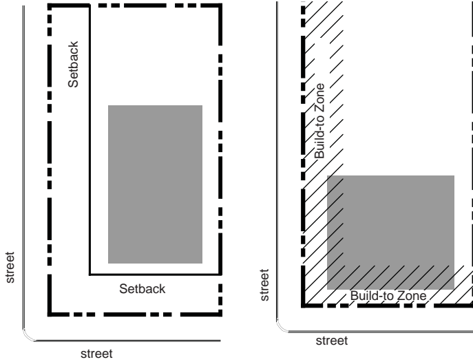
Figure 10.5 (2). Setback Line vs. Build-to Zone.
