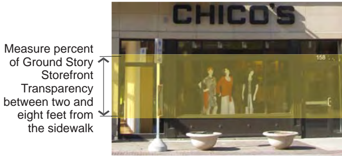
Measuring Ground Floor Transparency on a Storefront base.
