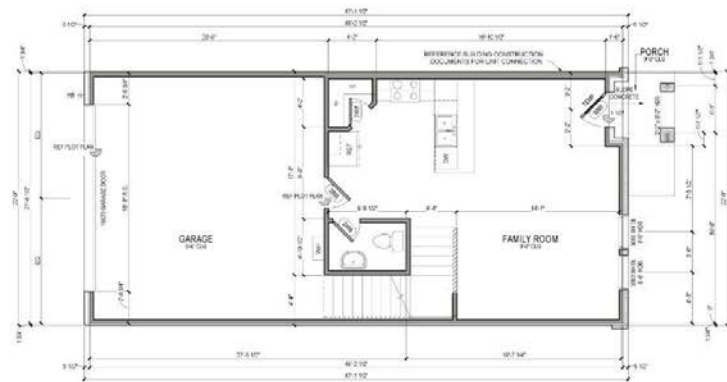
1 ELEVATION A - INTERIOR UNIT FIRST FLOOR PLAN
