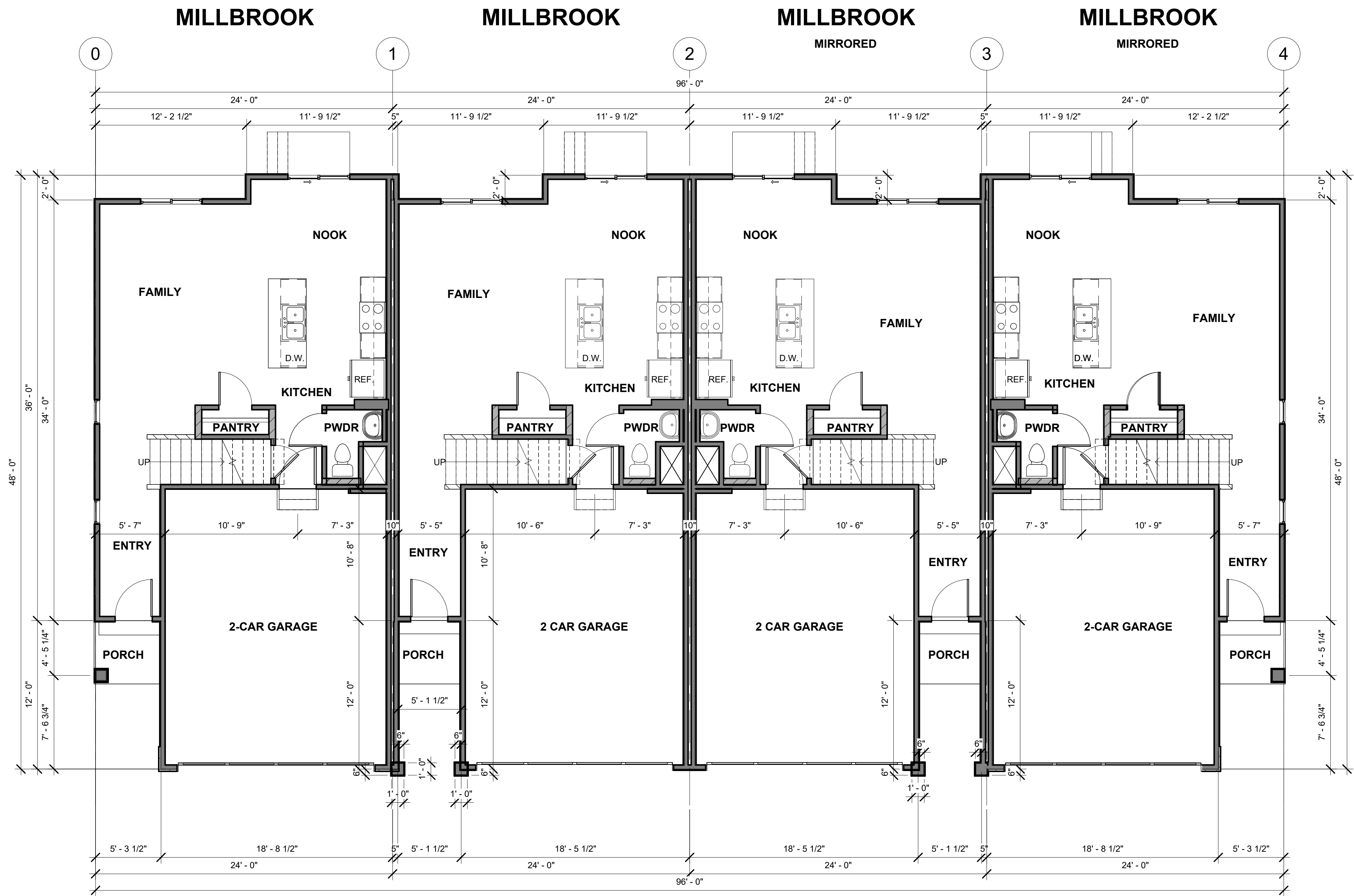
① TR - OVERALL FIRST FLOOR PLAN 3/16" = 1'-0"
