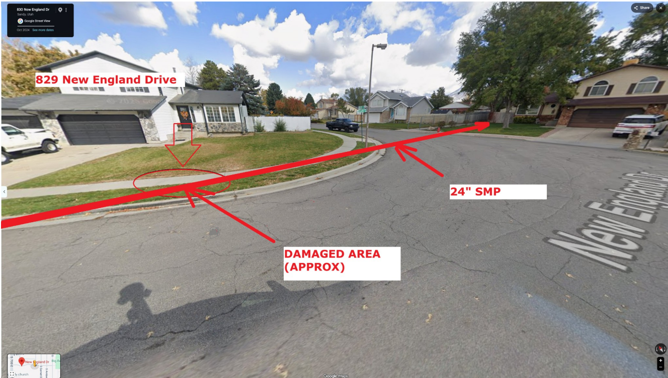
Street-level exhibit showing the approximate repair area and storm drain alignment.
