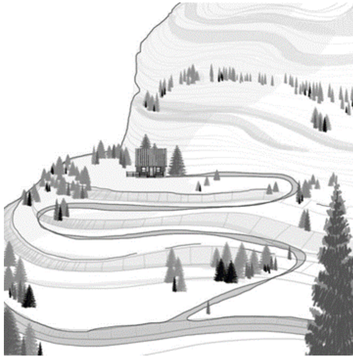
FIGURE 19.62.6: RECOMMENDED ACCESS ROUTE CONFIGURATION
