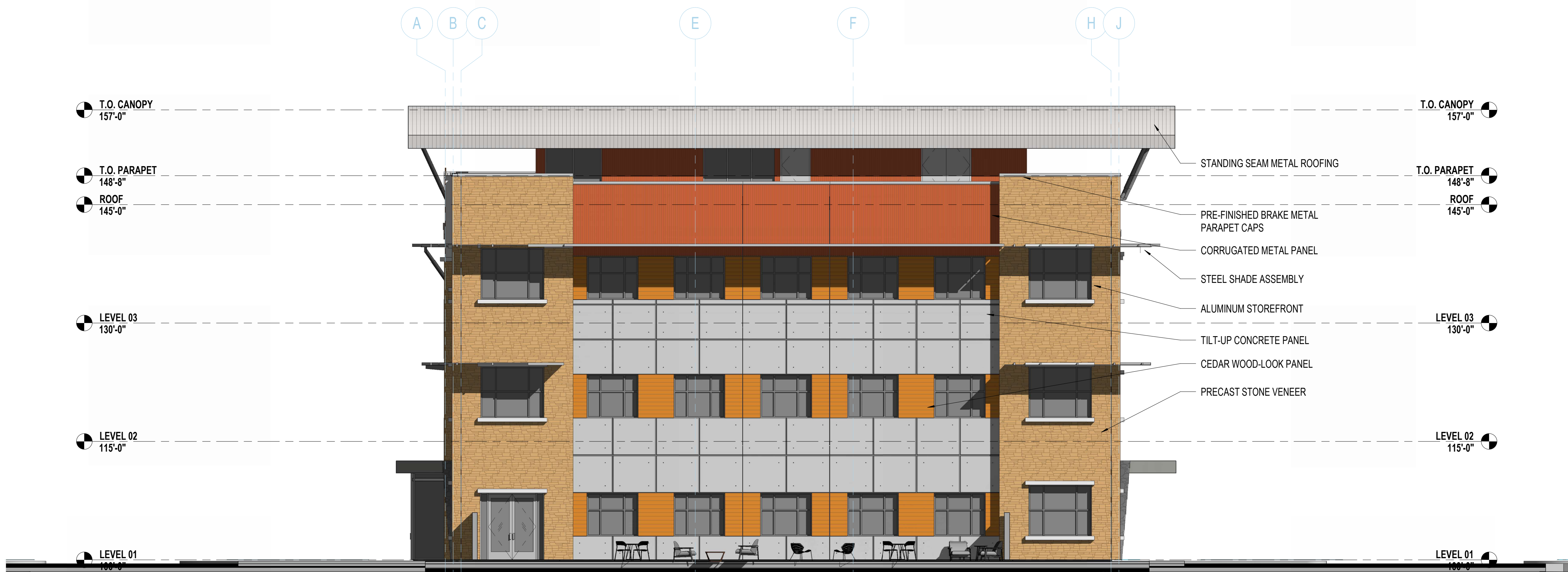
2 NORTH BUILDING ELEVATION A201 1/8" = 1'-0"
