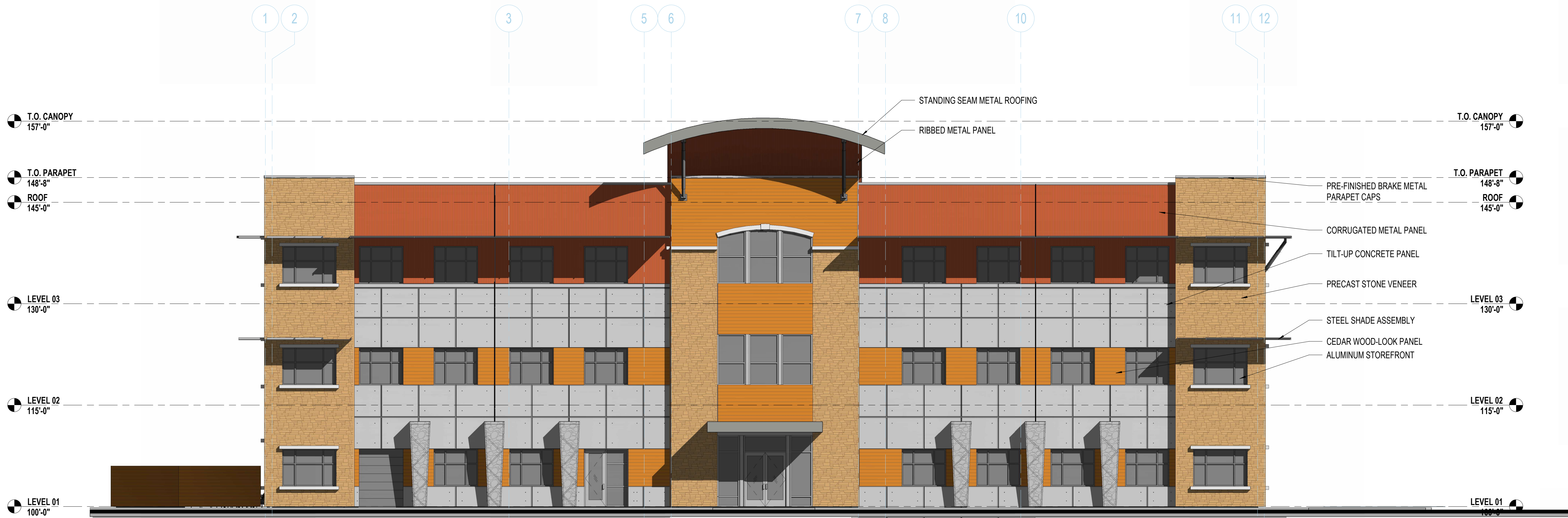
1 WEST BUILDING ELEVATION A201 1/8" = 1'-0"
