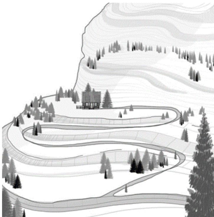
FIGURE 19.62.6: RECOMMENDED ACCESS ROUTE CONFIGURATION
