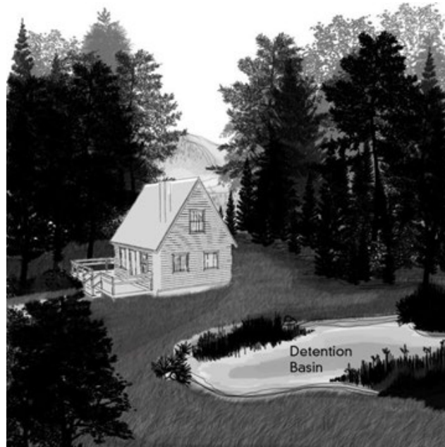
FIGURE 19.62.5: RECOMMENDED DETENTION BASIN TREATMENT
