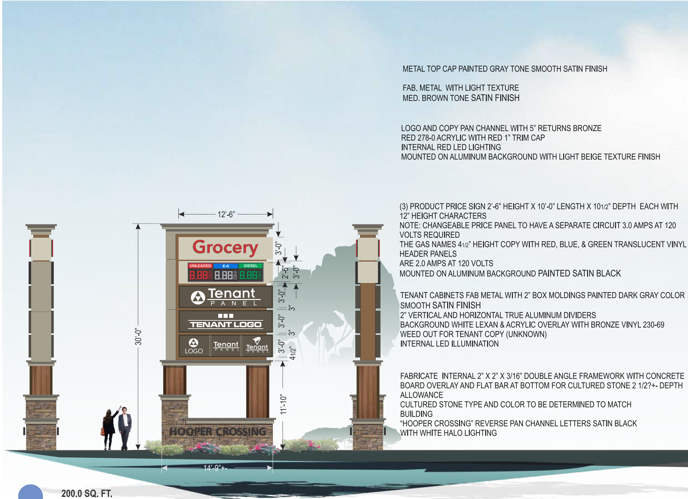
PYLON SIGN ELEVATION (4700 WEST STREET) SCALE: 1/8"=1'-0"
