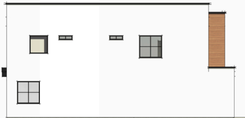
3 3 BED - 2 BATH LEFT ELEVATION 1/8" = 1'-0"
