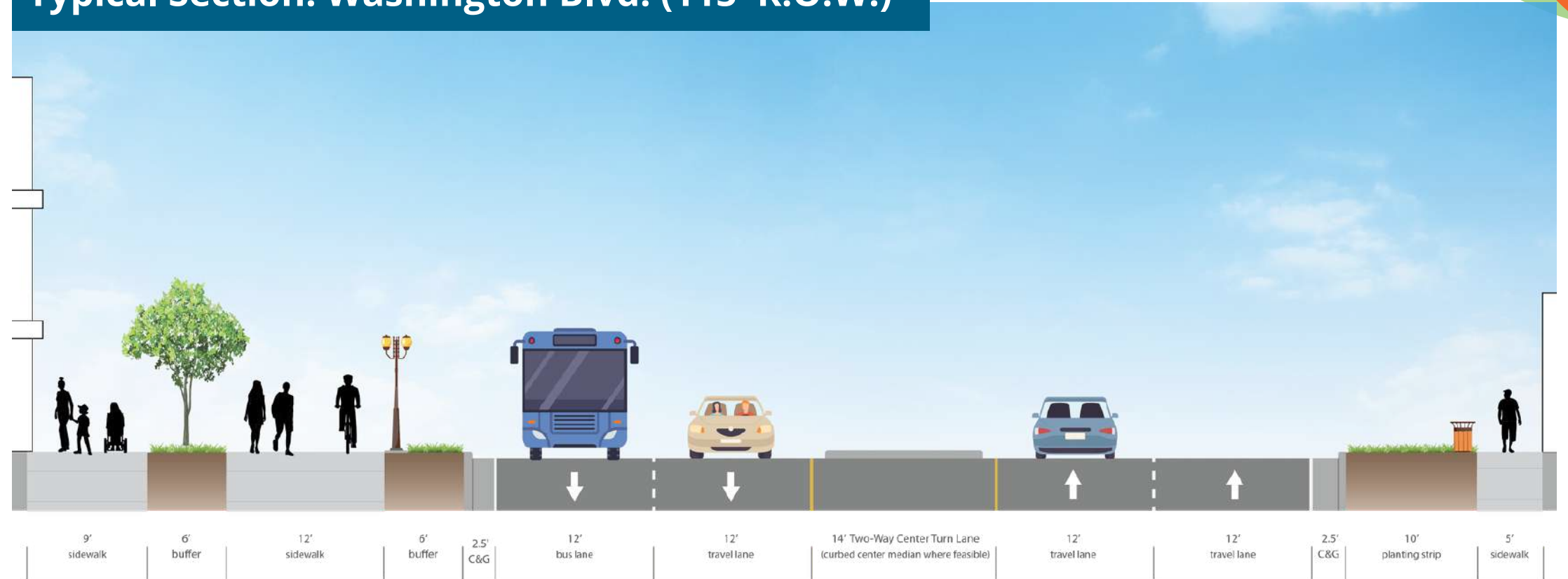
Typical Section: Washington Blvd. (115' R.O.W.)
