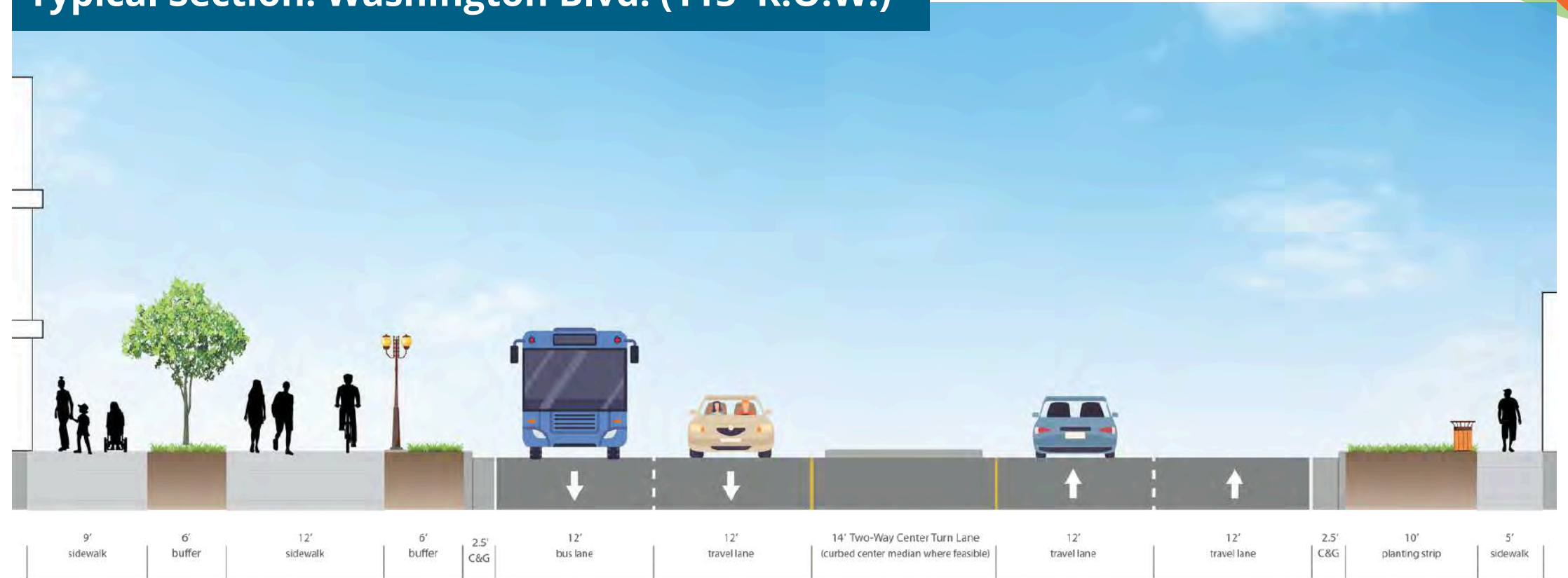
Typical Section: Washington Blvd. (115' R.O.W.)
