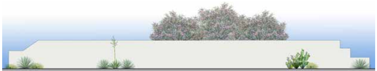
privacy wall; 6' stucco-clad masonry
