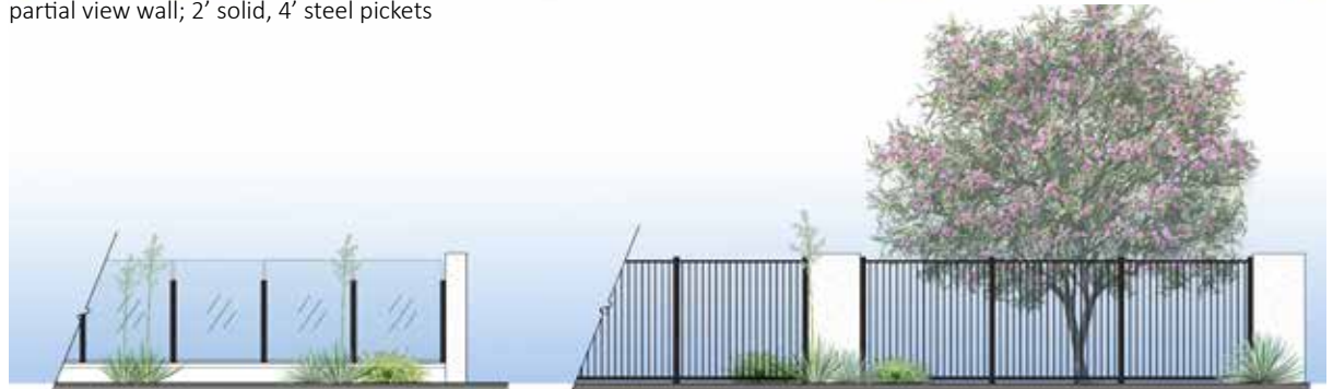
view wall; glass panels, steel posts
