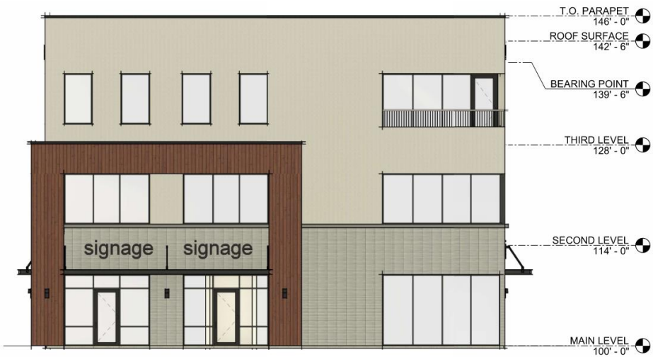
B1 LEFT ELEVATION 1/8" = 1'-0"
