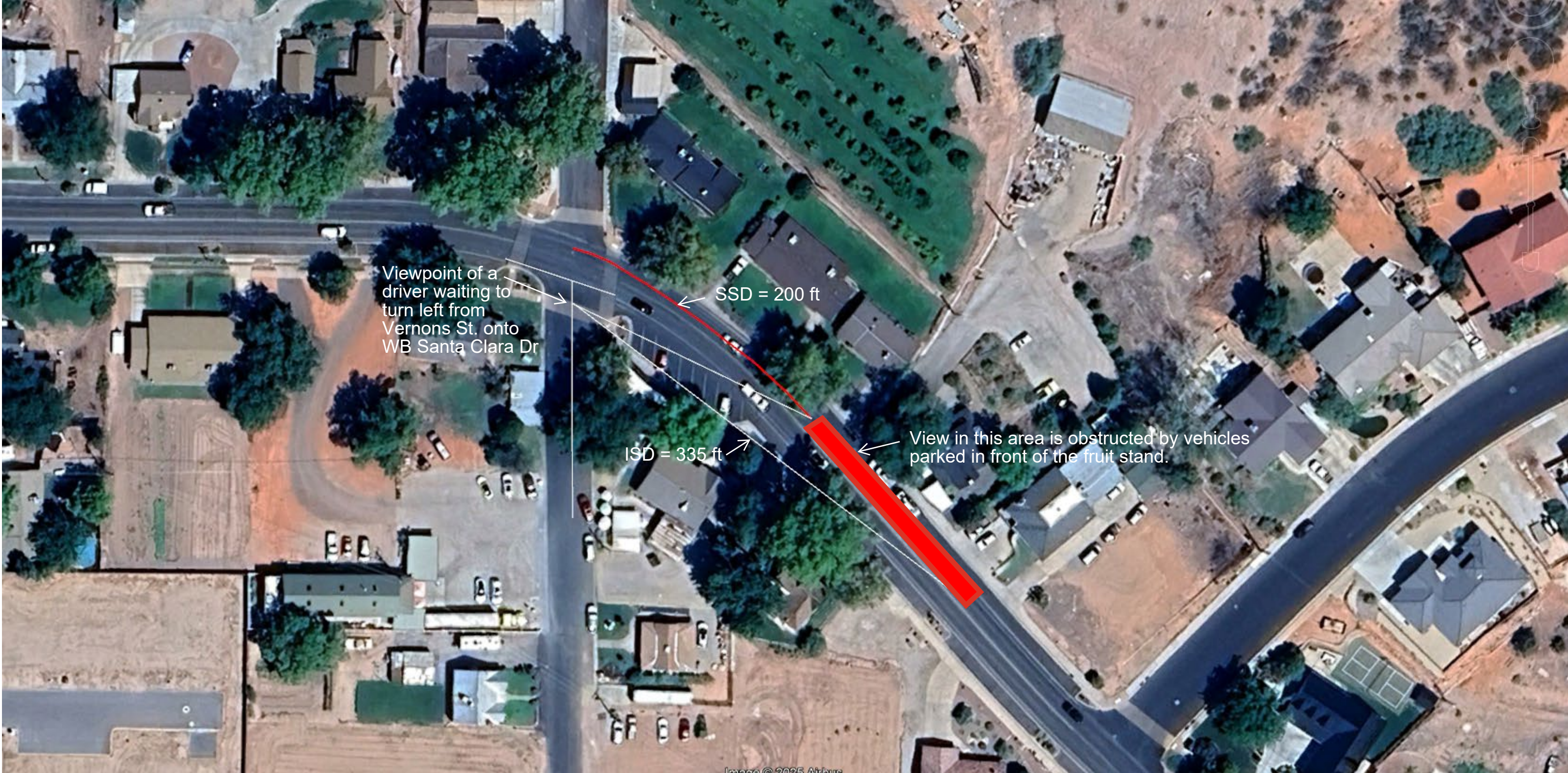
Stopping Site Distance (SSD) is the distance a vehicle traveling west at 30 MPH needs to stop to avoid a northbound vehicle turning left from Vernons St. Intersection Site Distance (ISD) is the required line-of-site distance published in the AASHTO design guideline for a 30 MPH street. The current width of the existing parking area could accommodate up to 3 parallel parking stalls (one of them being handicap accessible). Parallel parking still somewhat blocks the intersection site distance but it enables more site distance than diagonal parked vehicles.
