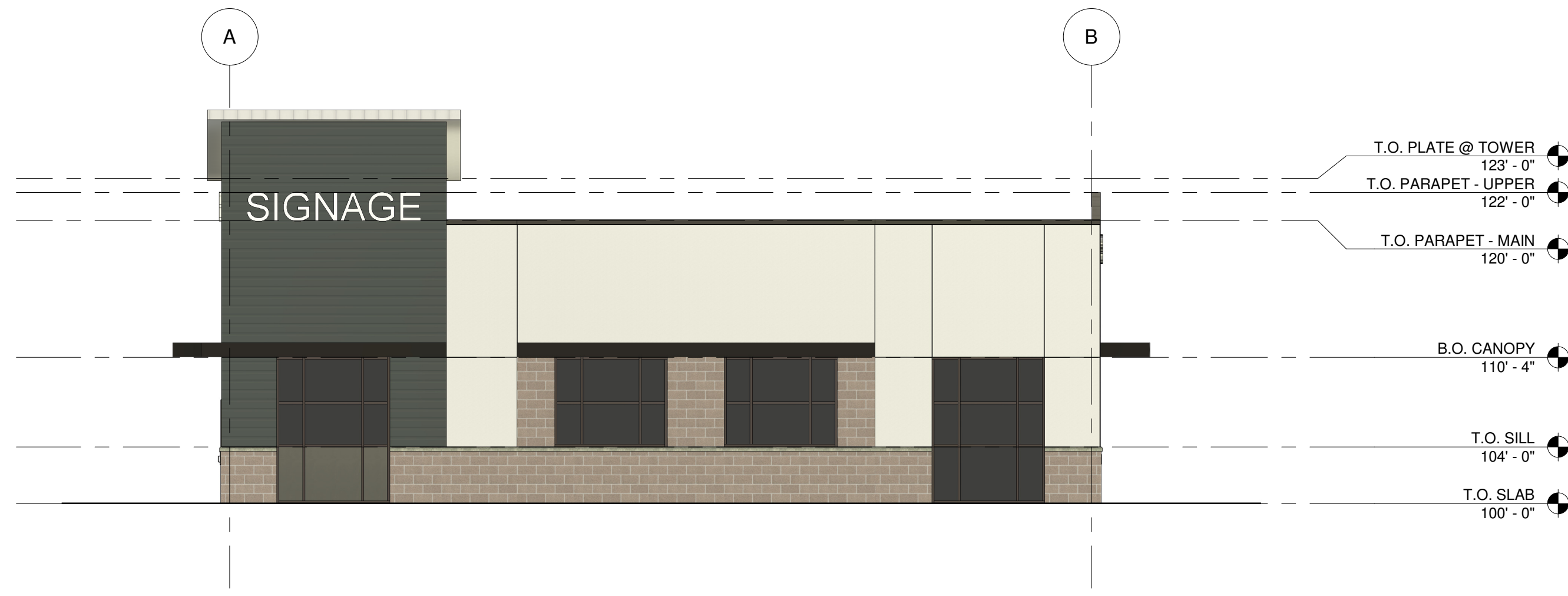
A CONCEPTUAL EXTERIOR ELEVATION - EAST (RETAIL) 1/8" = 1'-0"
