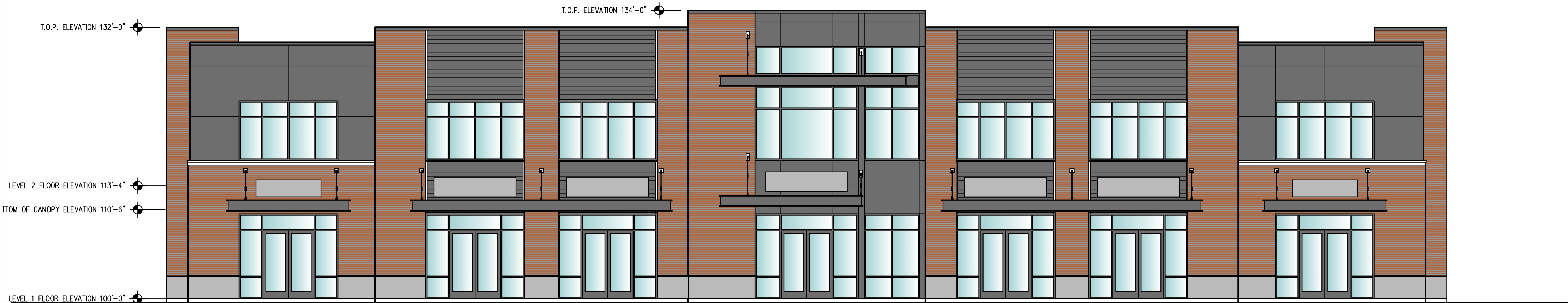
FRONT ELEVATION - SOUTH SCALE: 1/8" = 1'-0"
