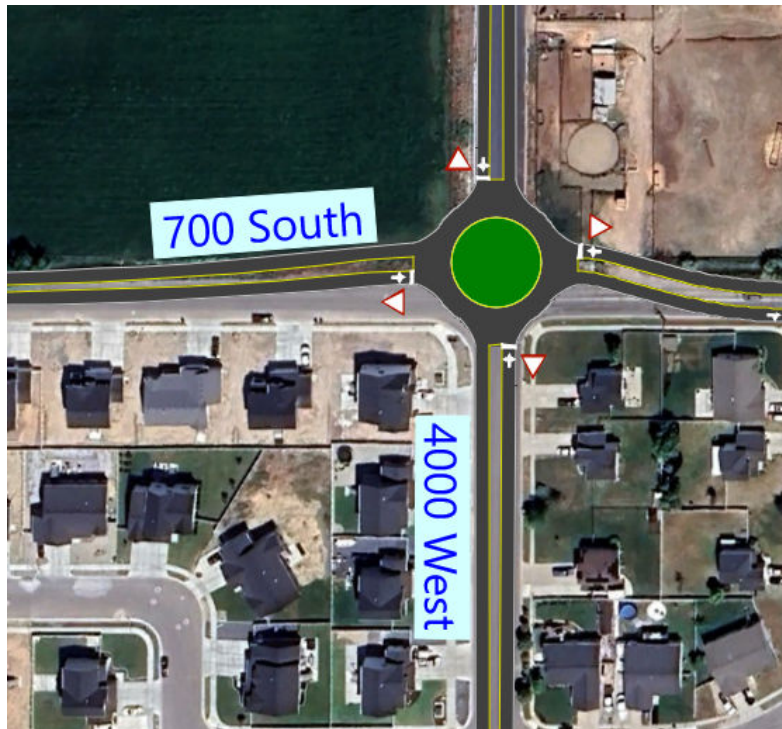
Figure 4: Roundabout Intersection Layout
