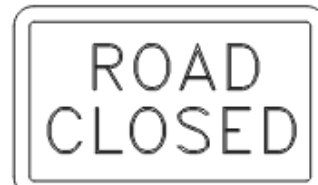
3 TYPE R11-2: ROAD CLOSED SIGN
