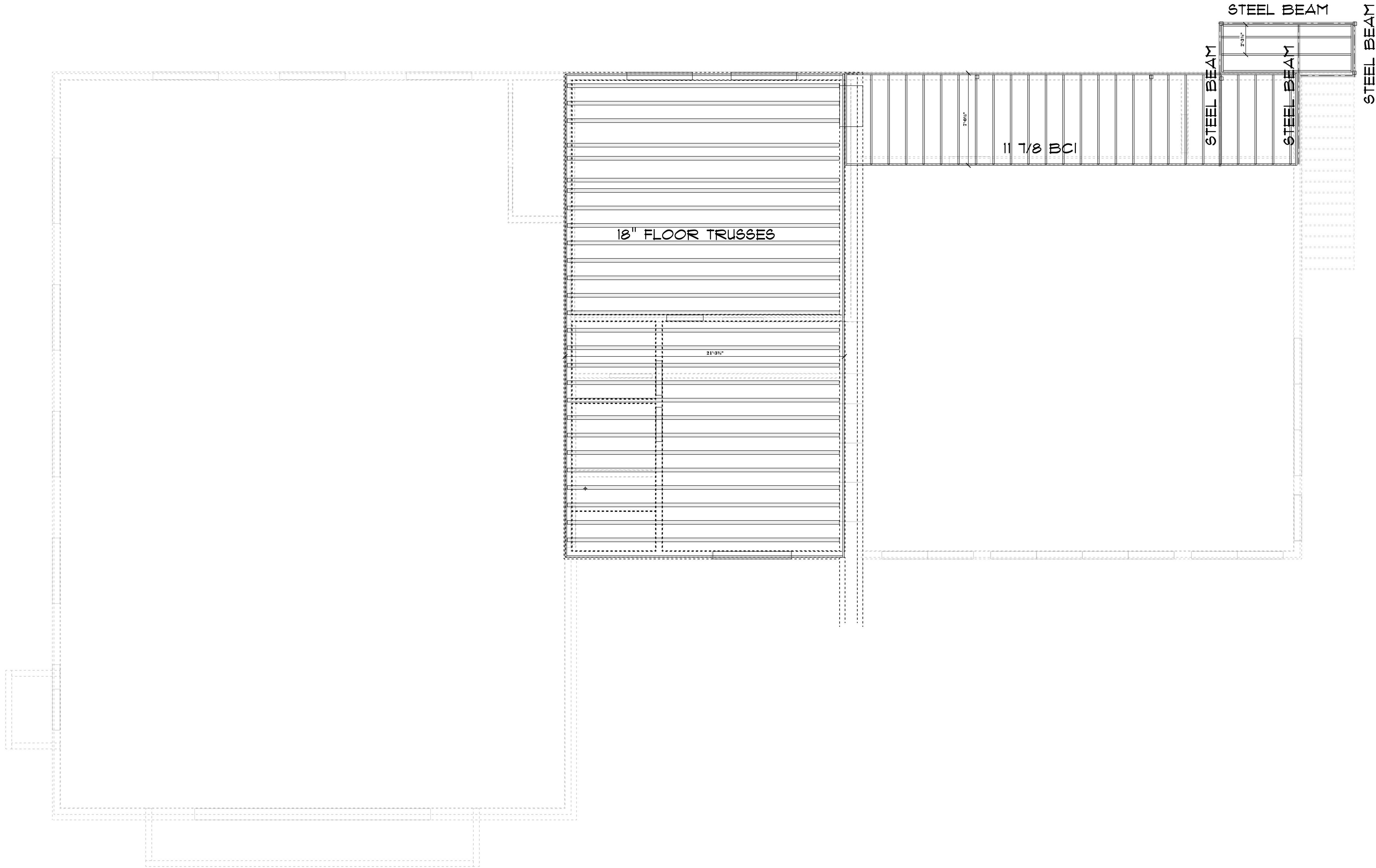
2ND FLOOR FRAMING - FLOOR SYSTEM SCALE: 1/4" = 1'-0"
