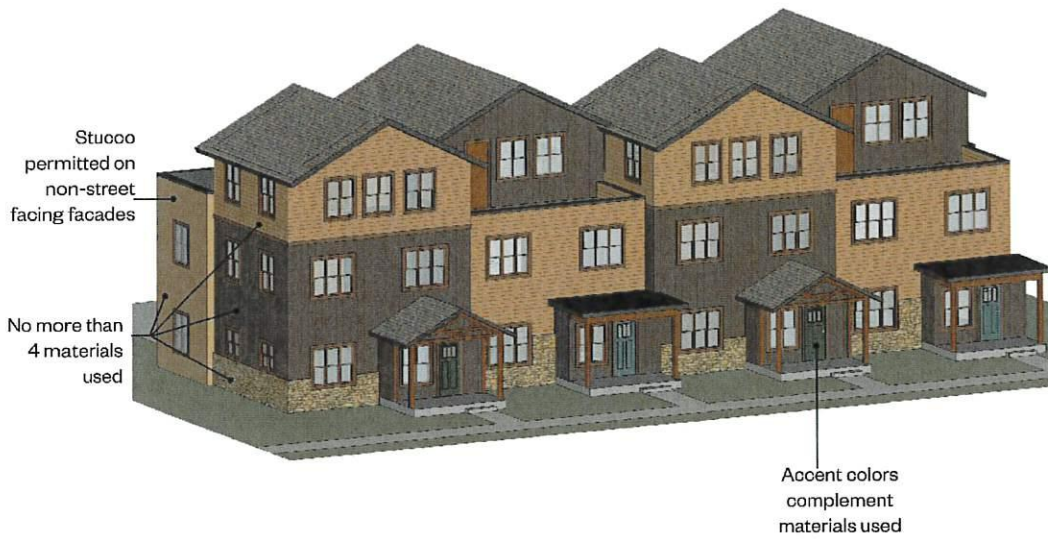
Multi-Family Building Materials with Alley Access Diagram.
