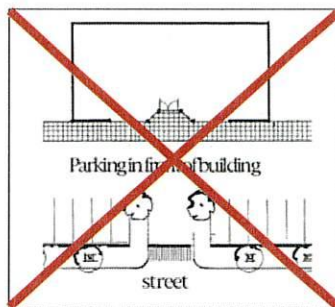
Not Permitted – Parking between building and street
