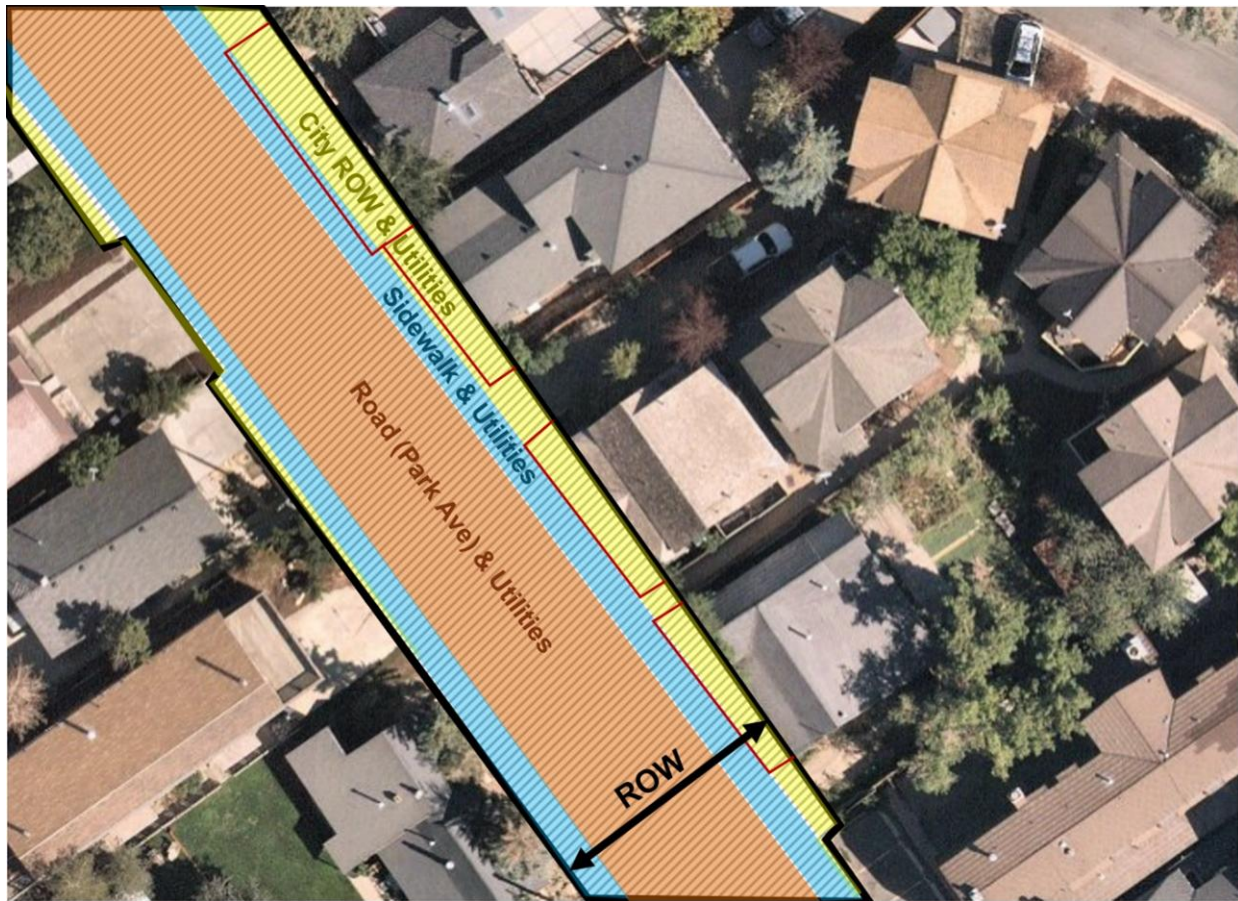
Figure 4: Excerpt from Nearmap of Park Avenue showing the ROW outlined in black, the Road highlighted in orange, the sidewalk highlighted in blue, additional ROW highlighted in yellow, and Fences in the ROW in red. Utilities are often found throughout the full width of the ROW.
