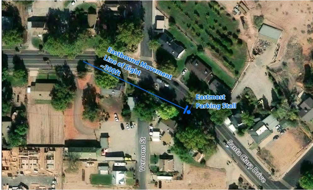
Figure 4: Stopping sight distance
