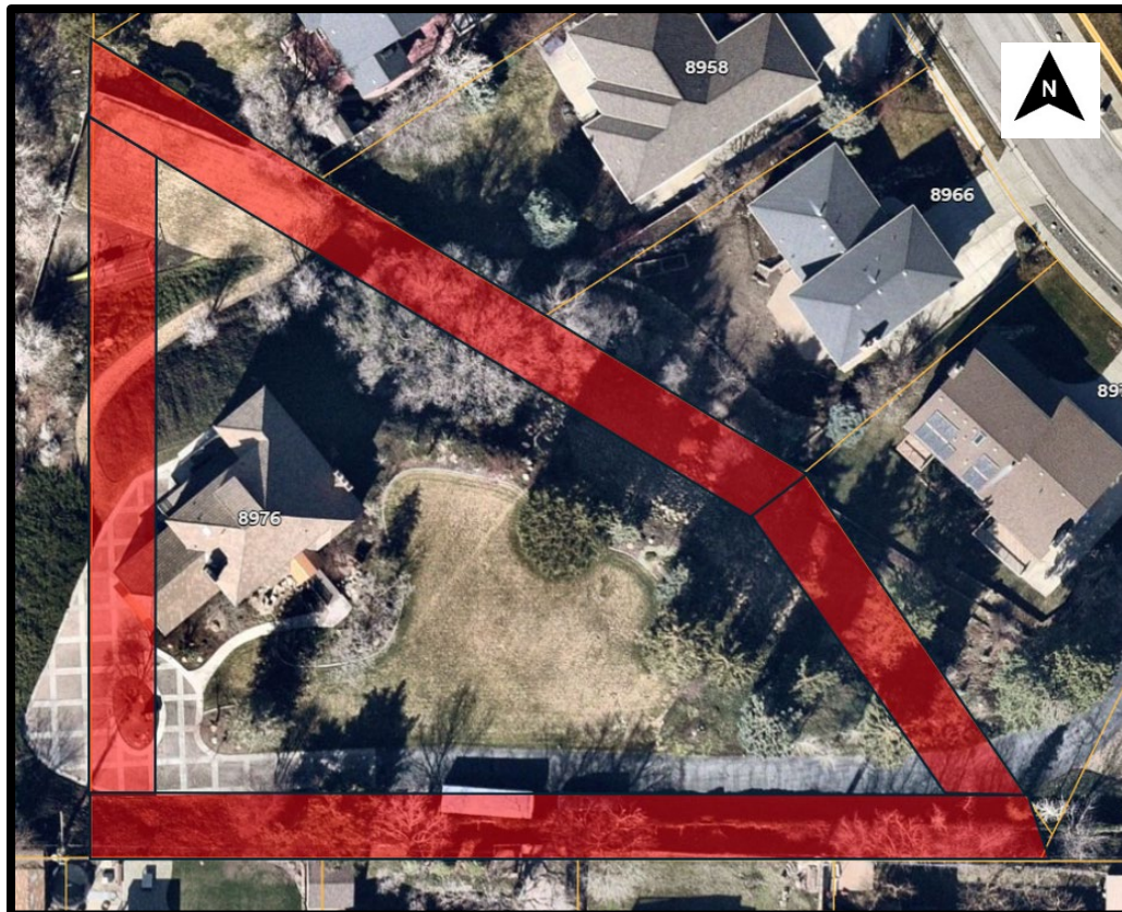
R-1-8 flag lot setbacks for the property (20-ft front, rear, and side setbacks)
