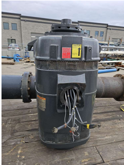
Vertical hollow shaft 250 hp motor
