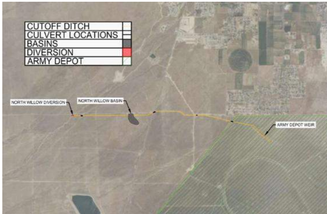
Figure 8-3: Existing Flood Protection Infrastructures
