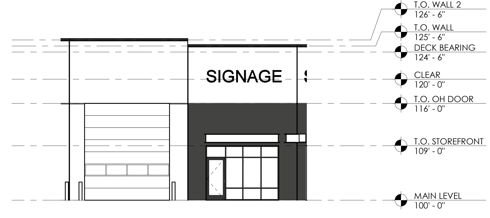
4 ENLARGED WEST ELEVATION - CORNER SIDE 1/8" = 1'-0"
