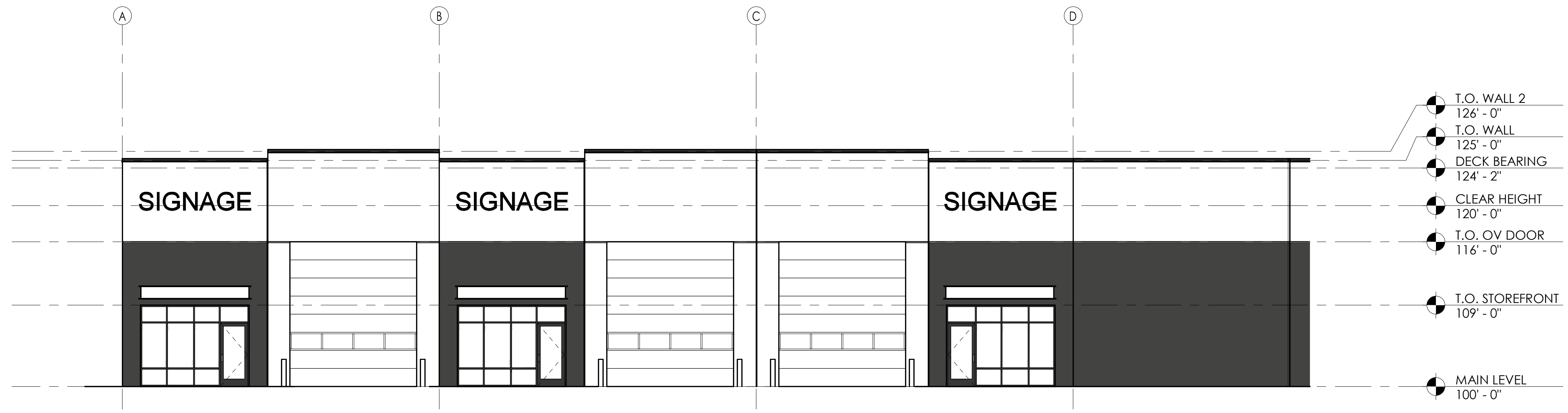
4 ENLARGED SOUTH ELEVATION - LEFT SIDE 1/8" = 1'-0"
