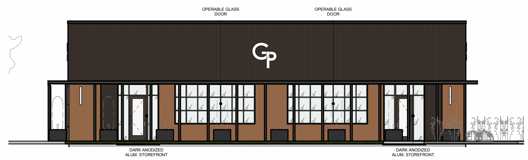
C1 A200 NORTH PAD A - EAST ELEVATION 1/8" = 1'-0"
