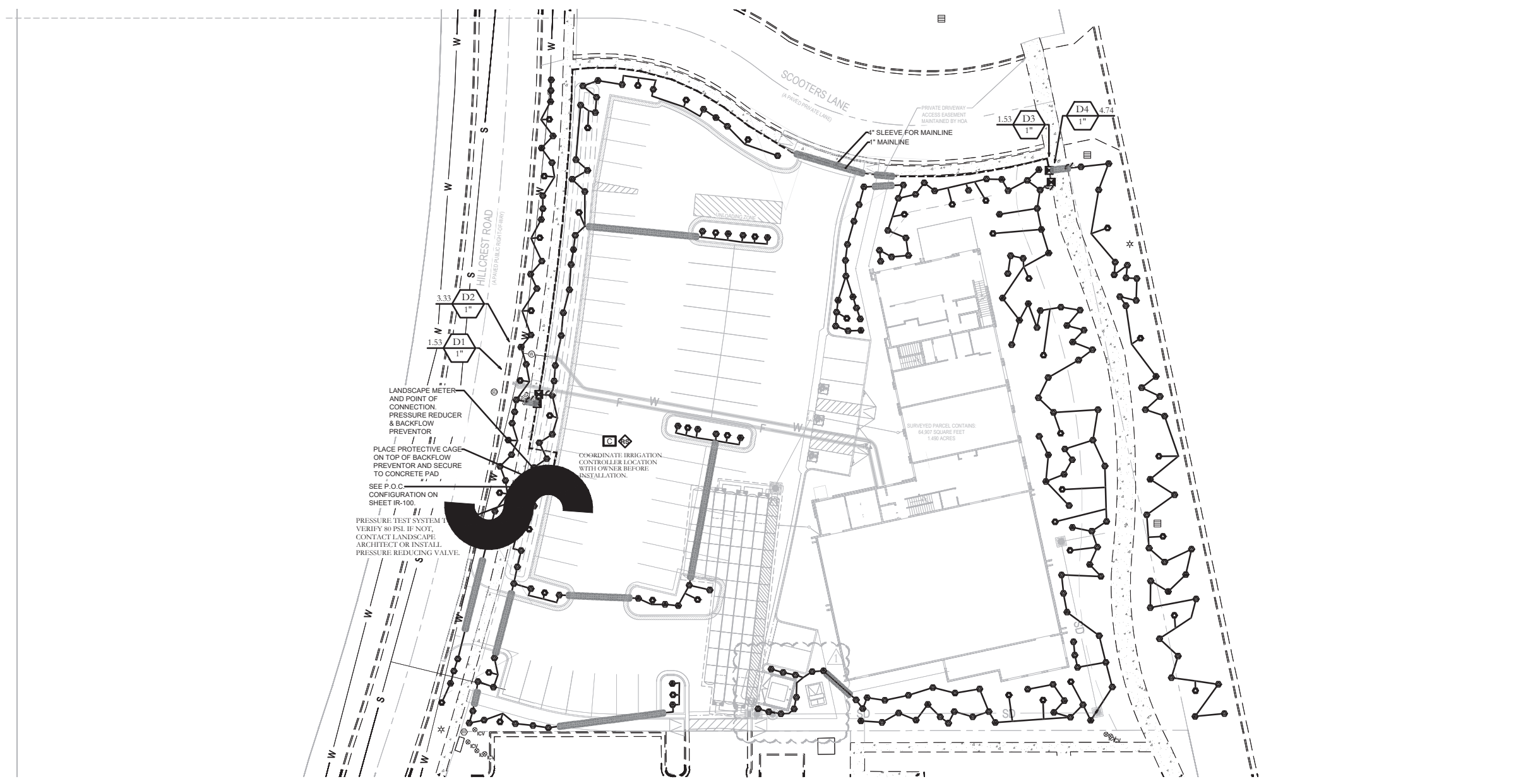
2" MAINLINE ROUTING, CONTROLLER AND P.O.C. LOCATION OVERVIEW
