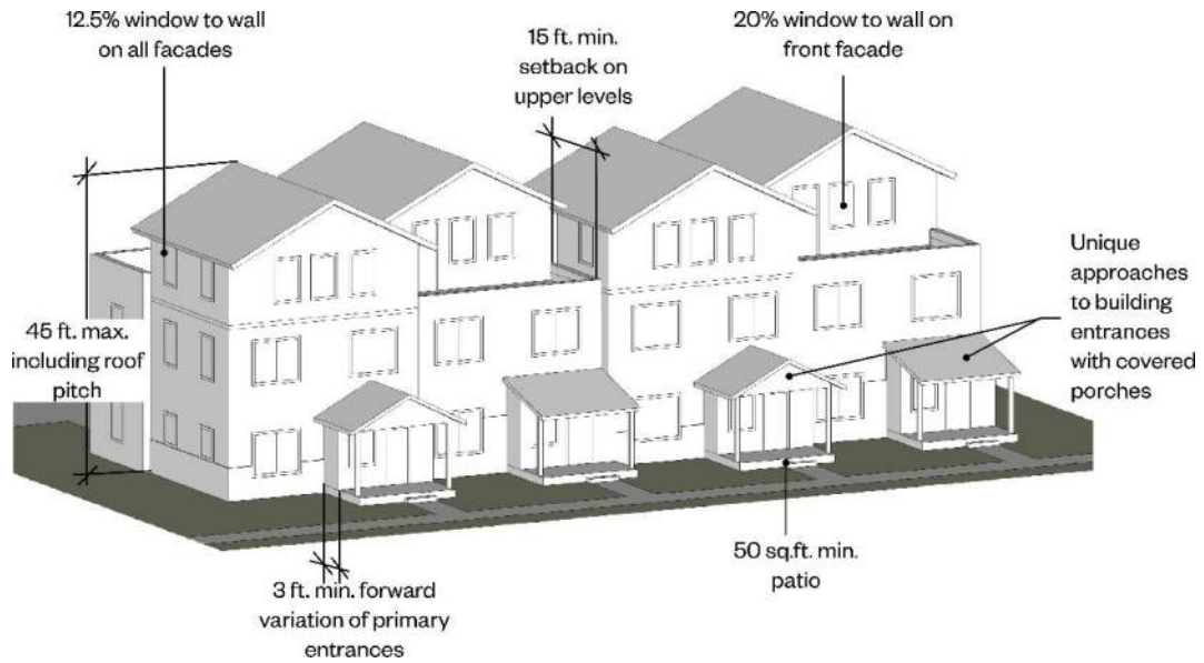
Multi-Family Building Height, Massing, Articulation, and Architectural Detail with Alley Access Diagram.
