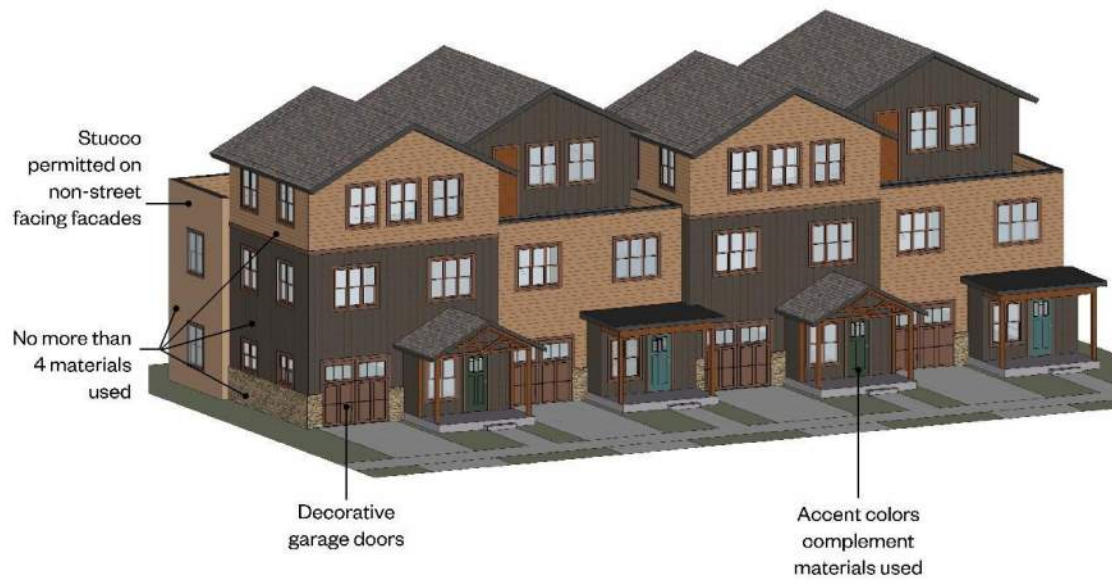
Multi-Family Building Materials with Front Garages Diagram.
