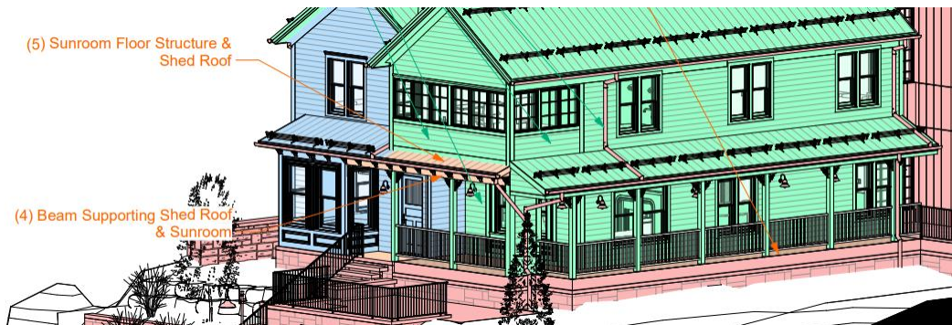
Figure 5: Applicant's proposed material deconstruction with items to be removed and replaced highlighted in orange.
