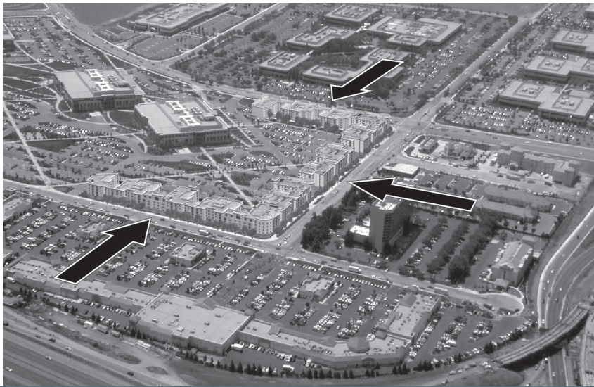
➔ Figure 3. The same office park from Figure 1, digitally altered to illustrate how removing parking requirements could result in liner apartment buildings on previously developed sites.
