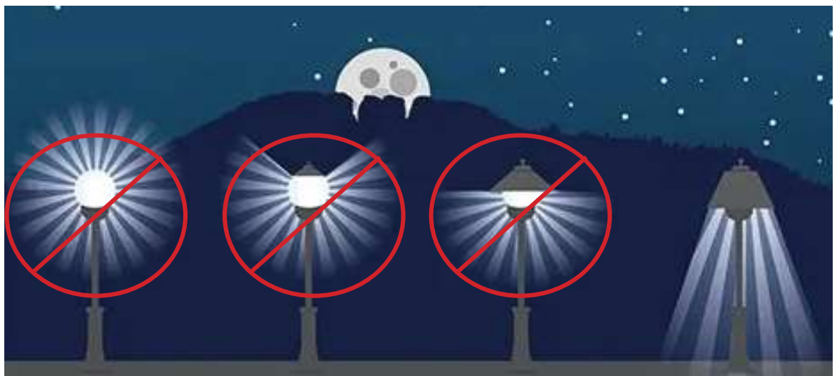
Figure 3.1 (1). Dark Skies Permitted and Not Permitted Fixtures
