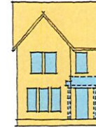
STEP 3: FACADE COMPOSITION Use the Pattern Book examples as a guide for locating windows, doors, and accent openings to create well-composed facades.
