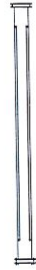
Square post with corner chamfer, simple base and cap 5.5"x5.5" Post* Min.
