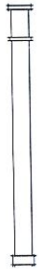
Square posts with simple cap, base trim, and astragal 5.5"x5.5" Post* Min.
