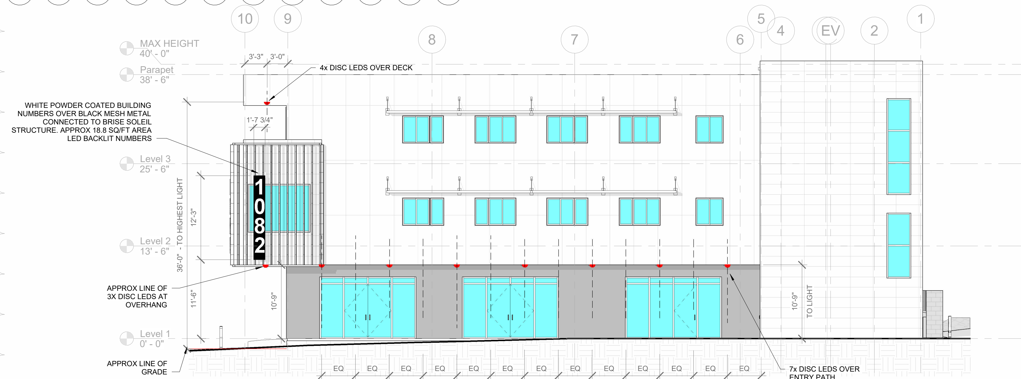
2 EXTERIOR LIGHTING BUILDING FRONT ELEVATION 1/8" = 1'-0"
