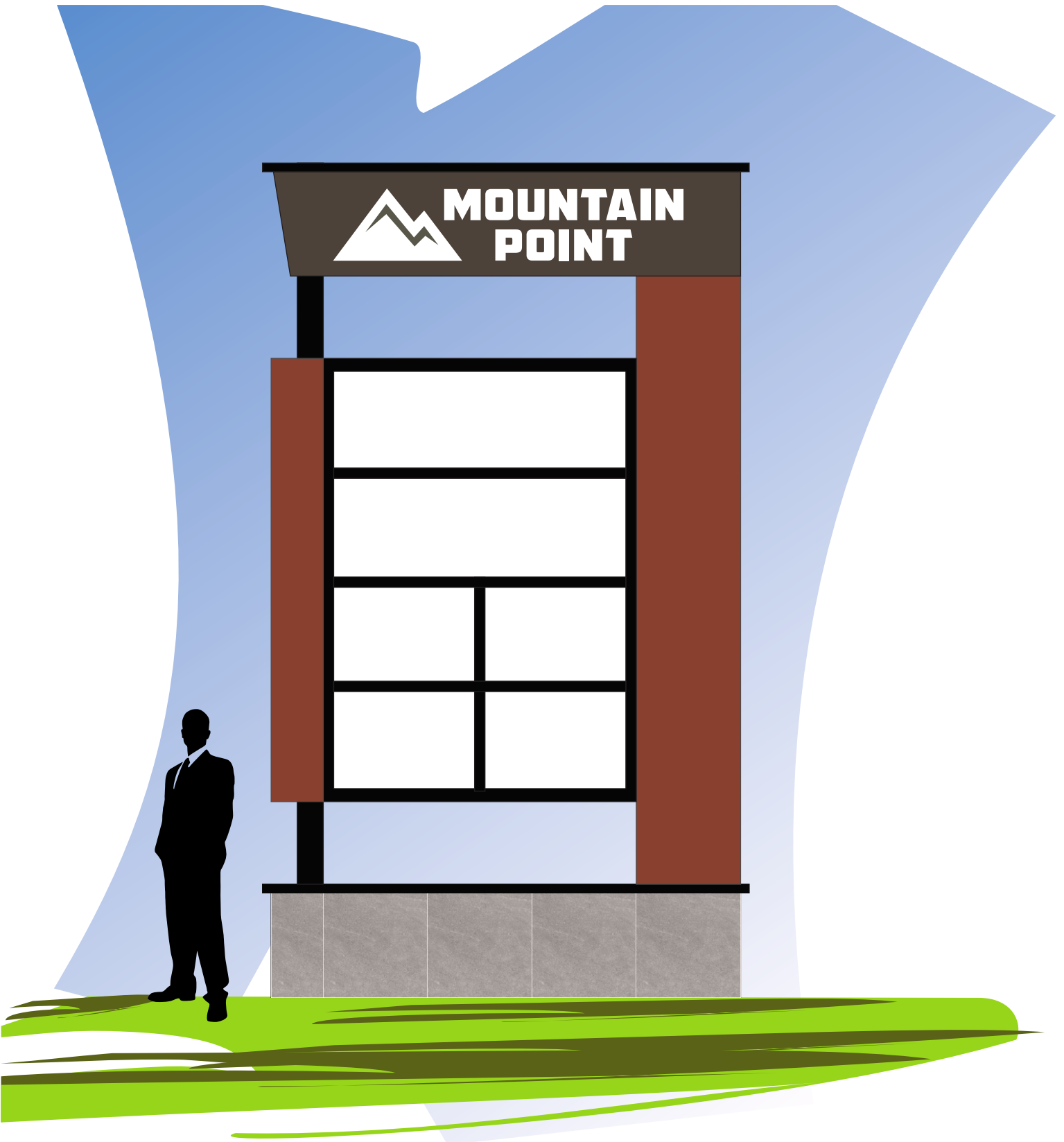
Pylon Sign: 16'-0" tall and 9'-4" wide (18" deep) Internally Illuminated Tenant Space Cabinet with 6ct. tenant spaces. "Mountain Point" cap piece is illuminated.
