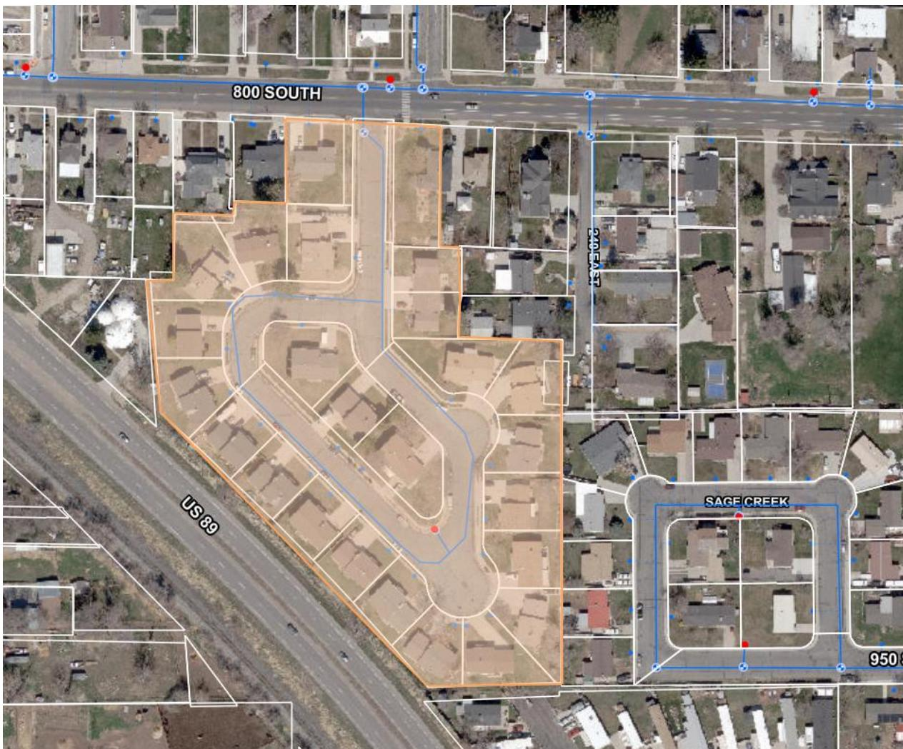
This Culinary Water Master Plan project will replace 6-inch diameter pipeline with new 8-inch diameter mains to assure fire-flow pressures, and add additional fire hydrants for better fire protection coverage.
